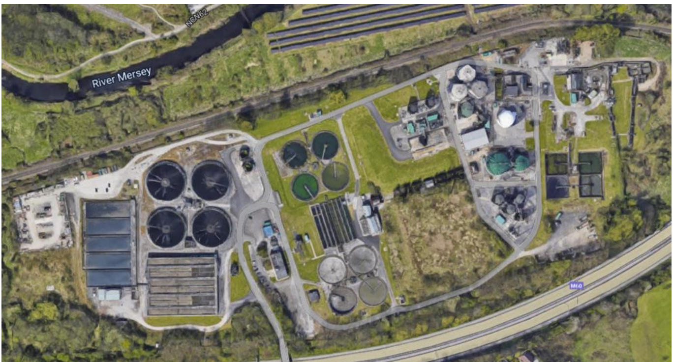
Figure 3: Stockport WwTW - Aerial photograph – Existing site layout
