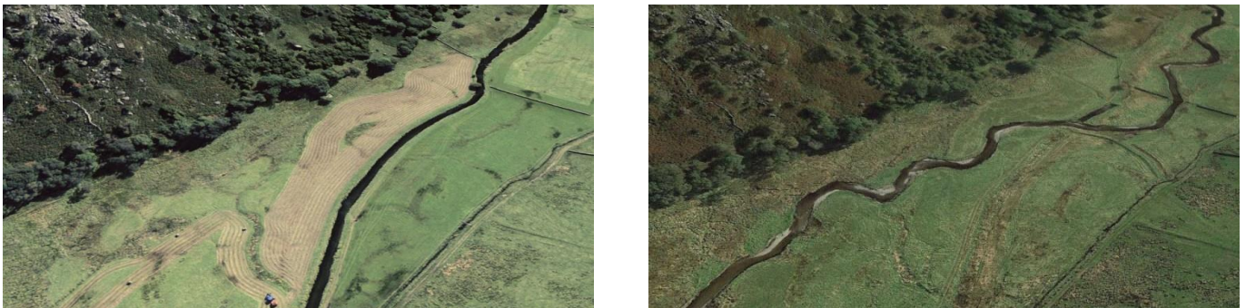
Figure 7: The re-meandering of Swindale Beck (shown before, on the left, and after, on the right)
