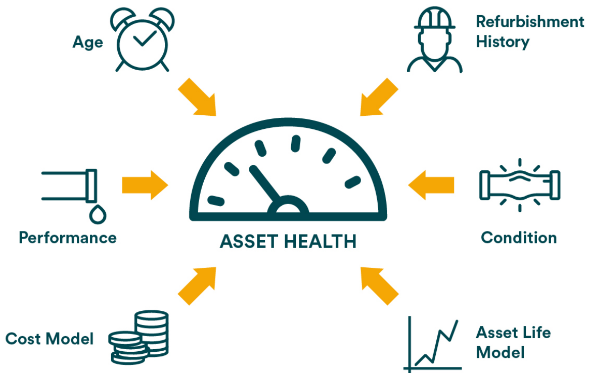
Figure 10: How existing asset health data streams feed into the Base Asset Health indicator
