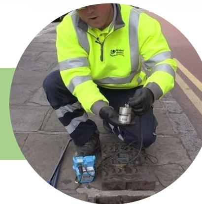
**Leakage: Acoustic loggers**
