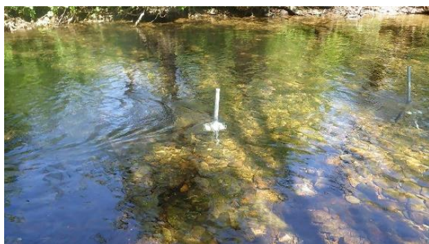
Figure 15 Installation of DGT (diffusive gradients in thin films) devices to monitor phosphorus in the River Ehen
