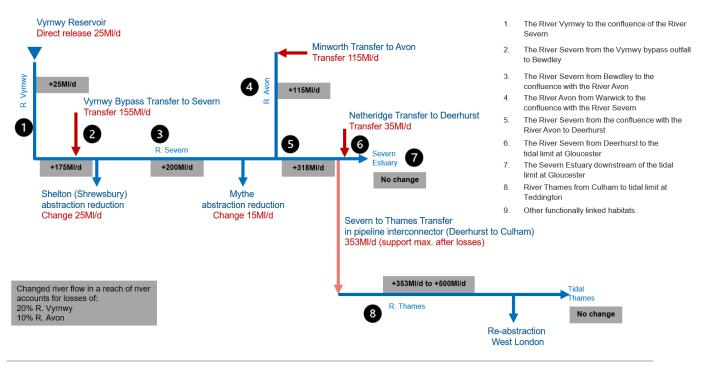
Figure 1.3 Schematic representing flow changes (accounting for losses) of STT Solution.
