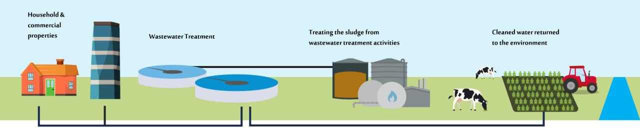
We take it away: what you flush down the loo and pour down the sink, along with rainwater drained from streets, goes through a network of sewers to one of our 500+ wastewater treatment works. We clean and return it: the wastewater is cleaned and returned to lakes, rivers and the sea.
