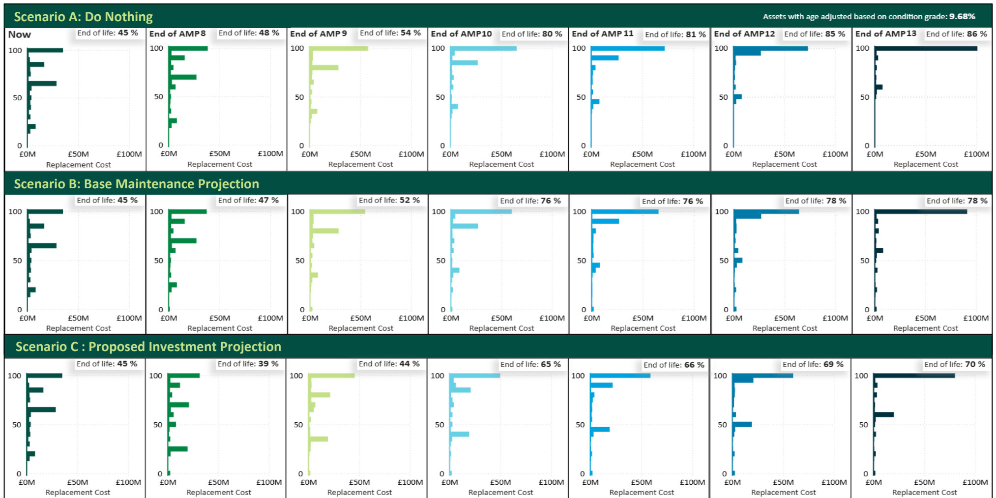
Figure 8: Scenario A – Asset health profile with no investment in borehole assets & Scenario B – Asset health profile with UUW’s current AMP8 plan and Scenario C – Asset health profile with UUW’s current AMP8 plan, plus the investment in this case
