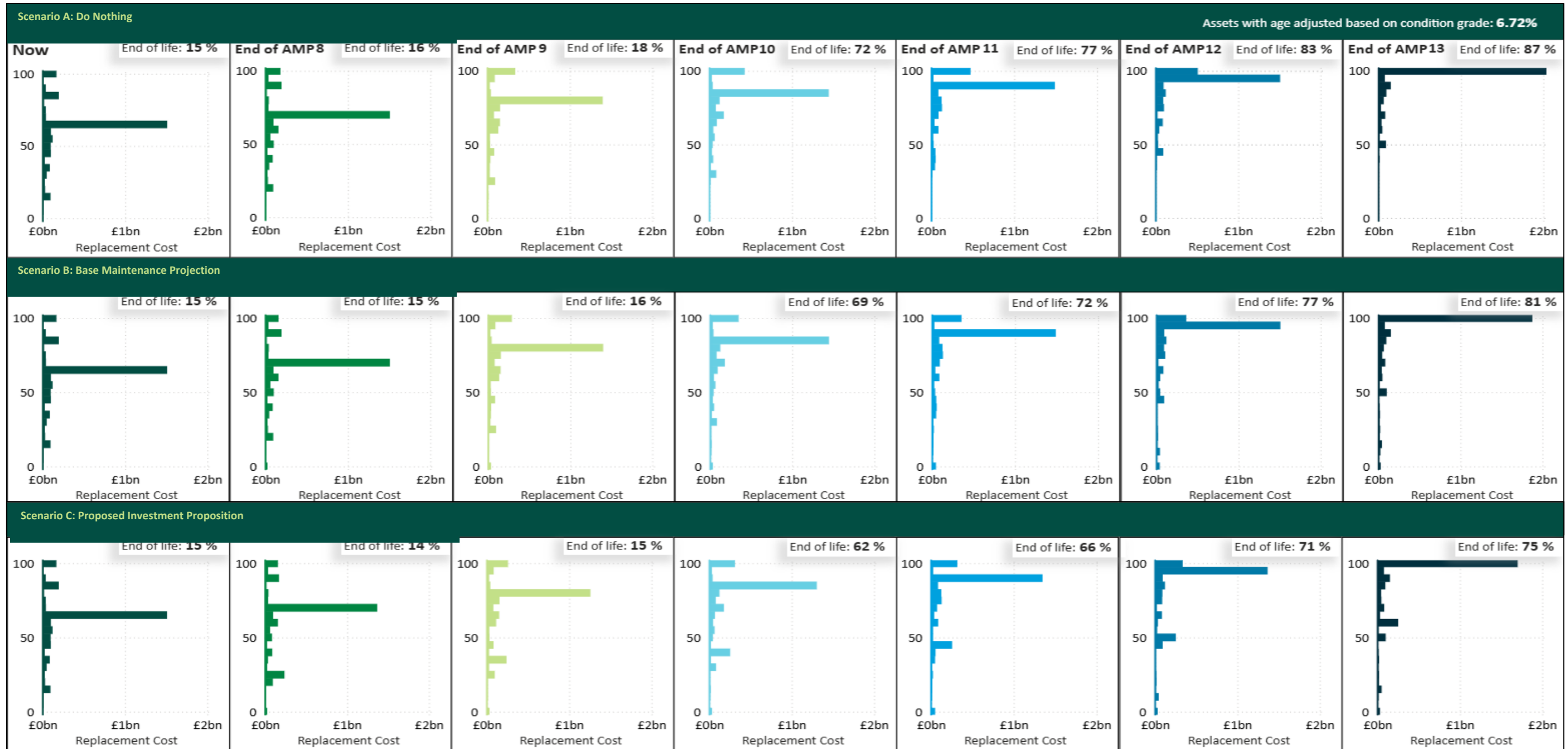
Figure 6: Scenario A – Asset health profile with no investment in treated water storage assets.; Scenario B – Forecasted asset health profile with AMP8 investment and Scenario C – Forecasted asset health profile with AMP8 investment and this business case.
