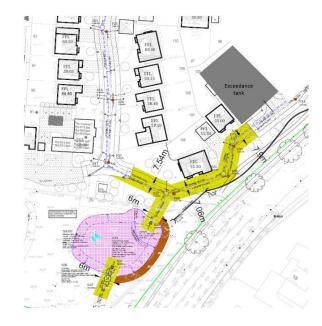
Inline Detention Basin (Discharging to surface water sewer)
