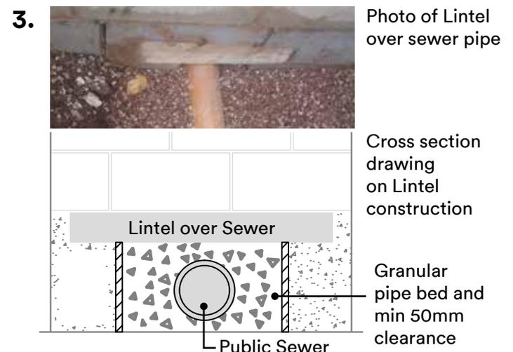
Cross section through foundations and sewer showing protective measures
