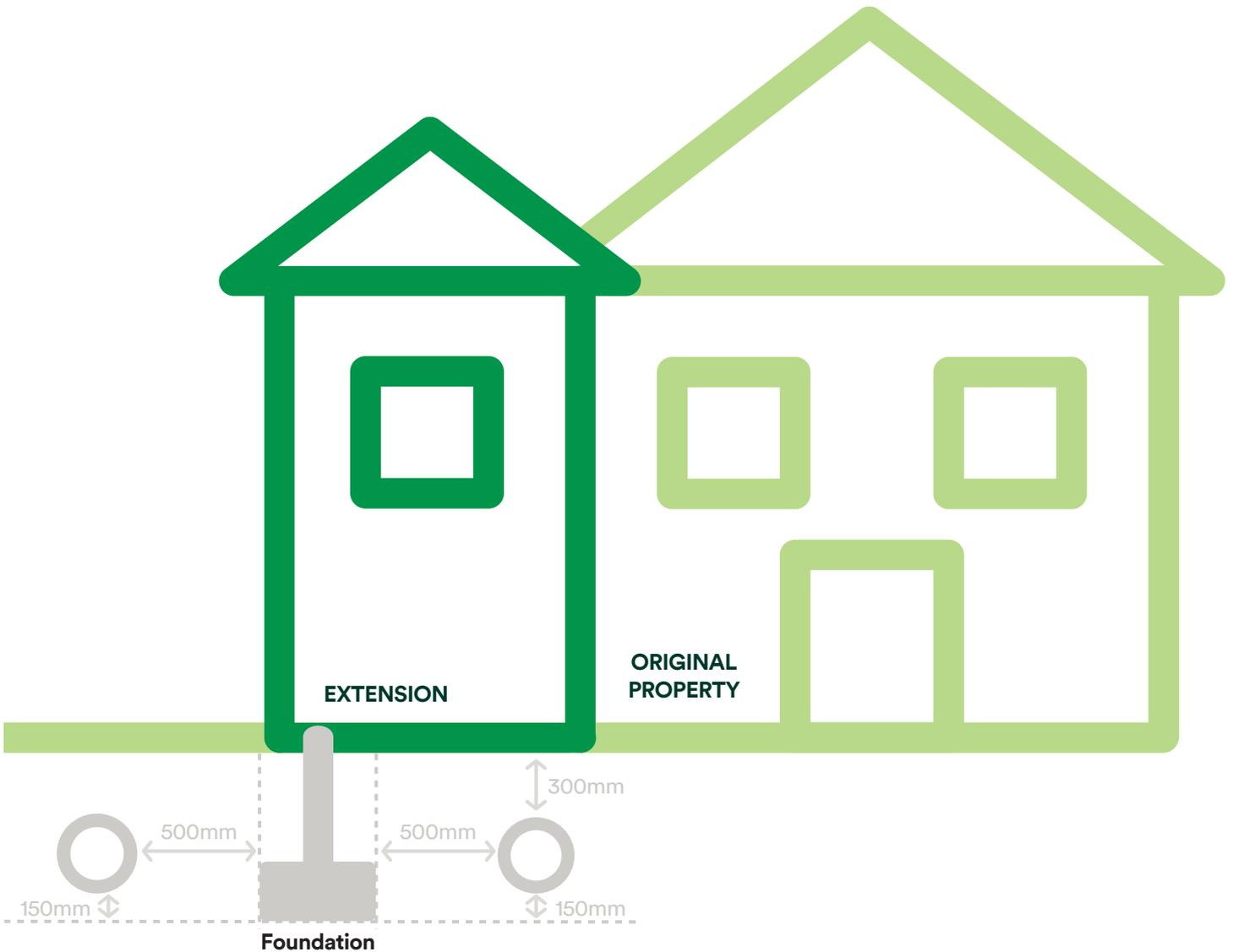
Minimum 500mm horizontal clearance between foundation and sewers.
