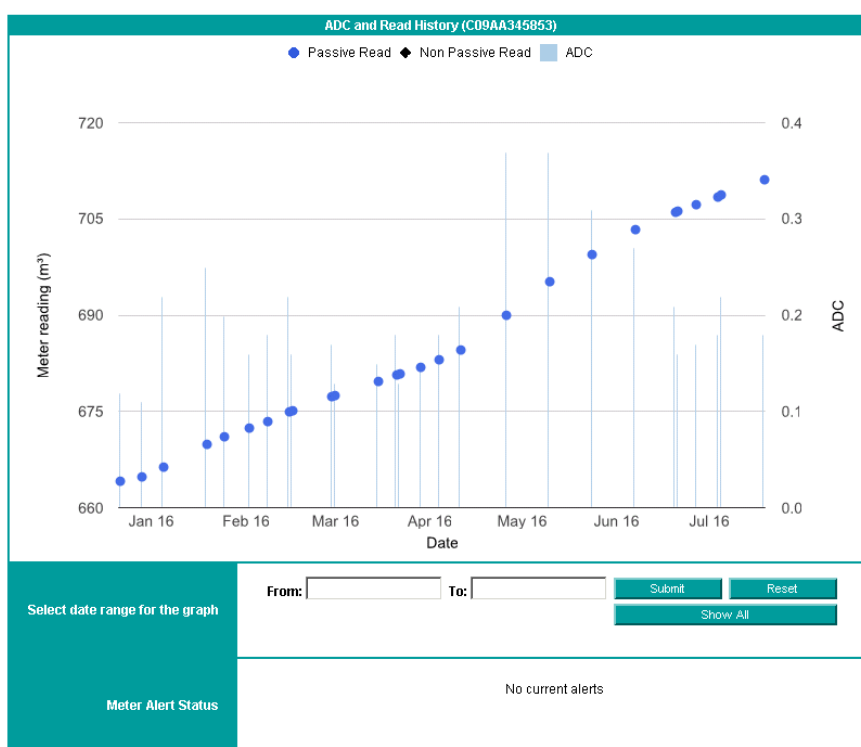
Figure 9 AMR portal – example screenshot
